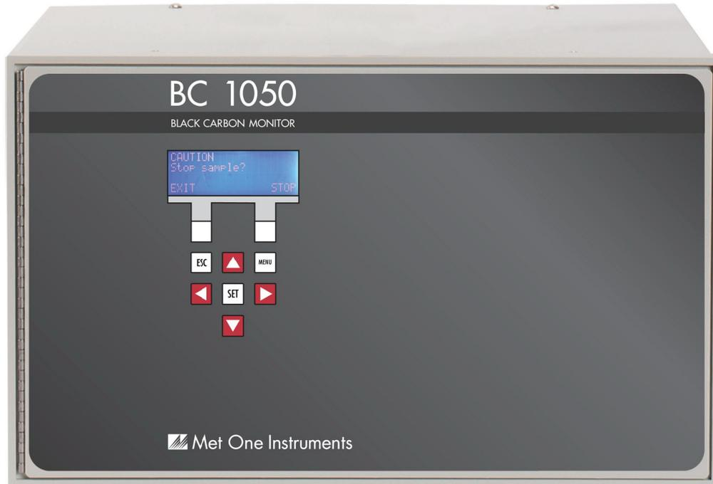
**The Met One Instruments BC-1050 Black Carbon Monitor** measures black carbon through optical attenuation and absorption principles in both the infrared and ultraviolet spectral regions. The BC-1050 offers improved traceability for the measurement of black carbon (BC) compared to traditional filter-based optical techniques through its unique factory calibration process and through the incorporation of standard EPA-style sampling inlets.
